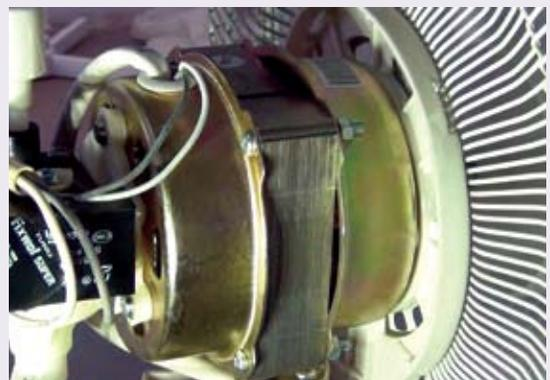
Close-up of motor and oscillation assembly of a typical pedestal fan
