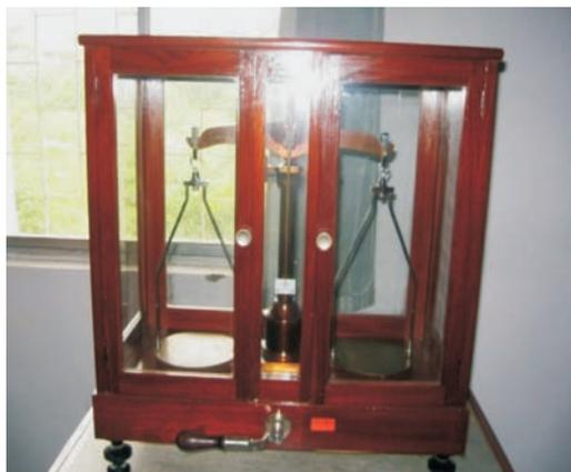
*Working Standard equi-arm double pan balance in Working Standard Laboratory*
