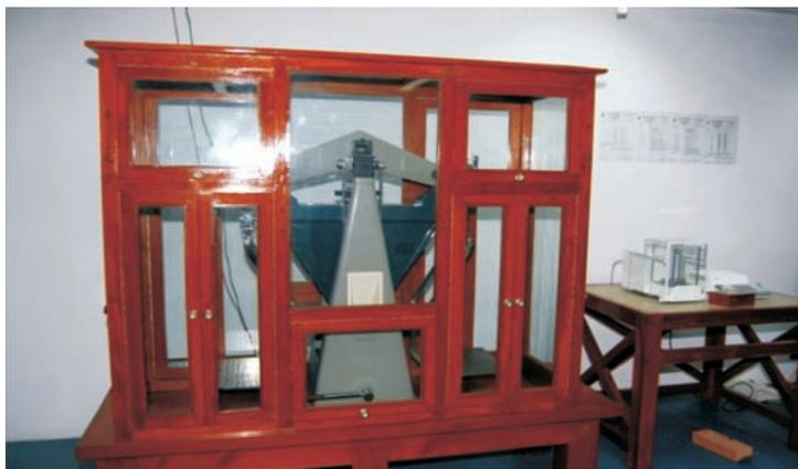
*Reference Standard equi-arm double pan balance in reference Standard Laboratory*
