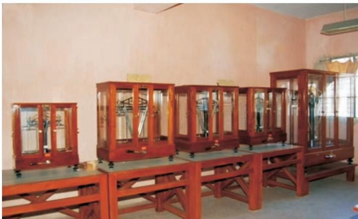
*Secondary Standard equi-arm double pan Balance in Secondary Standard Laboratory*
